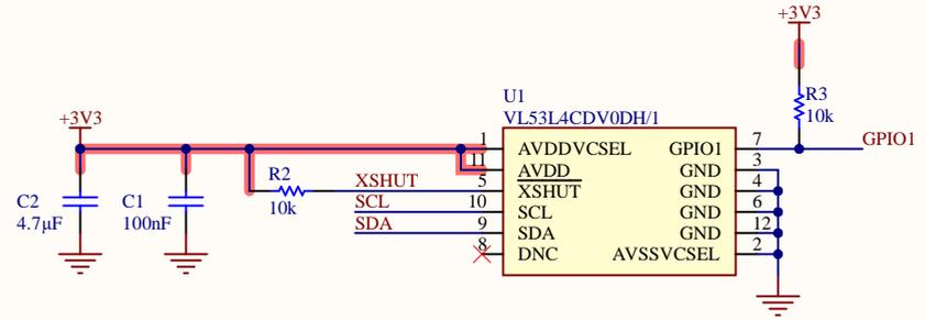
GPIO1 is open drain
