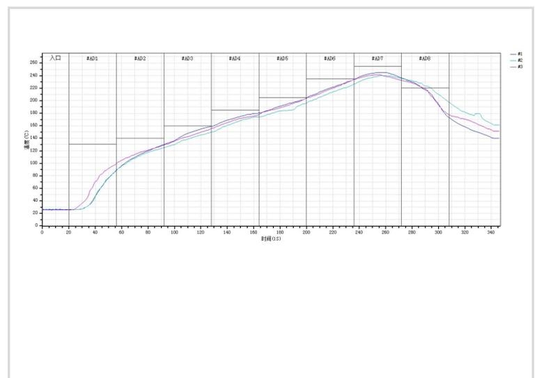
Remarks: 1. All the above temperatures refer to the temperatures measured on the surface of the package body
