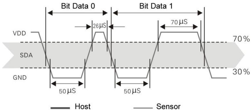
Figure 8 Single Bus Decomposition Sequence Diagram
