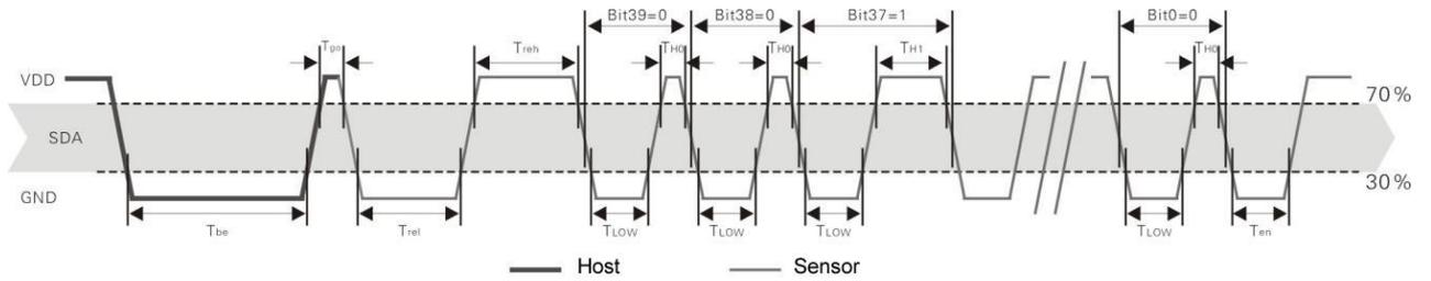
**Figure 6** CM2122 Single bus communication timing
