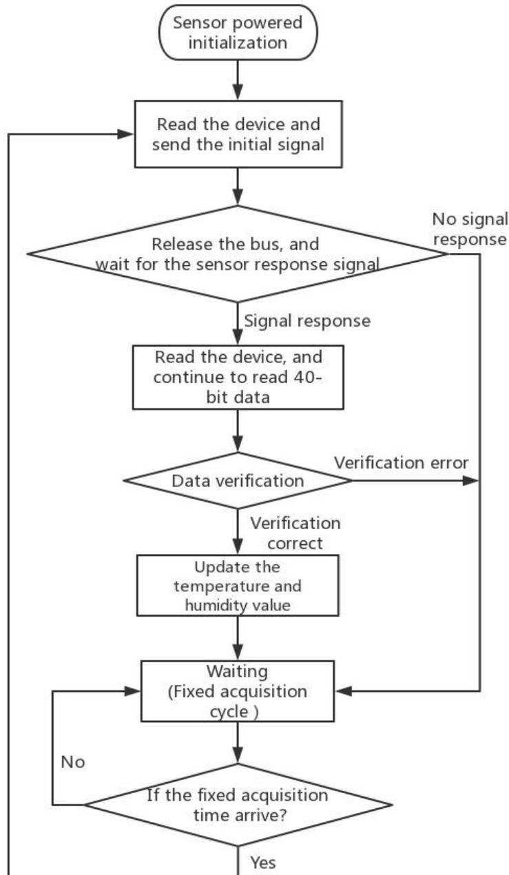
Figure 9 The Single Bus Read Flow Chart
