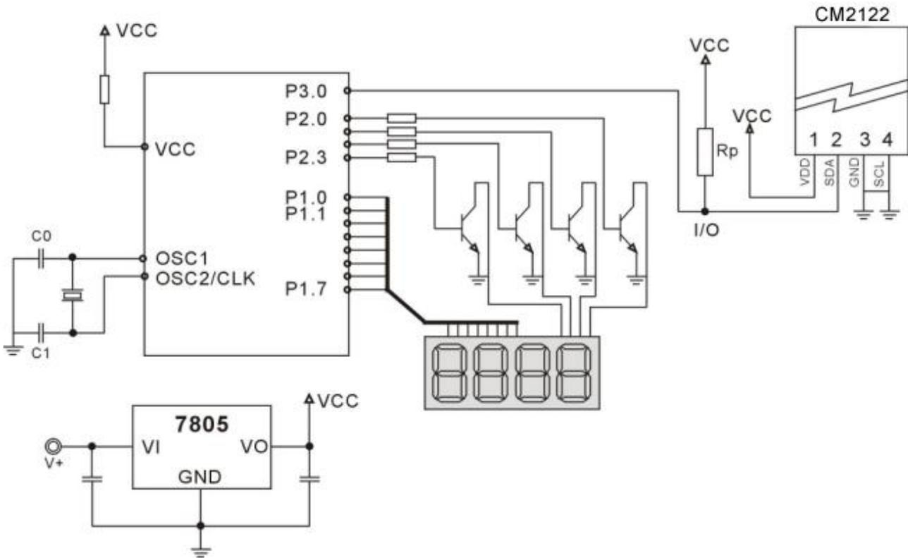
Figure 4 CM2122 One-Wire Application Circuitry
