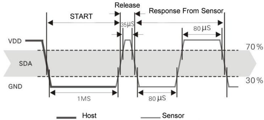
Figure 7 Single Bus Decomposition Timing Diagram
