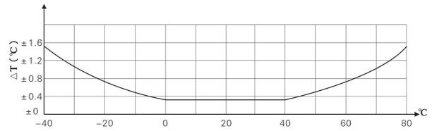
Figure 3 Typical Temperature Accuracy
