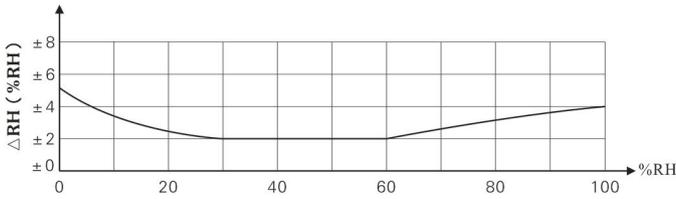
Figure 2 Typical RH% Accuracy at 25°C
