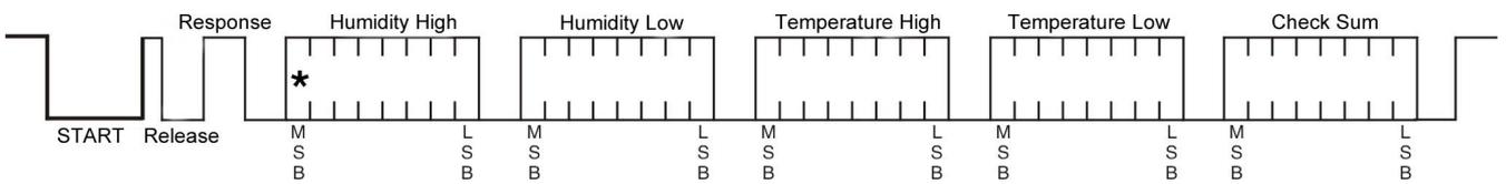
Figure 5 CM2122 Single Bus Communication Protocol
