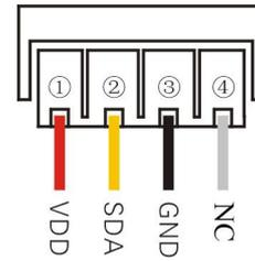
Figure 4 CM2122 Wiring Diagram
