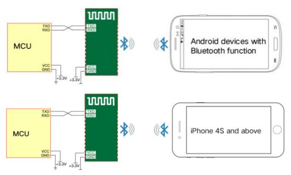
HC-42 supports connection to and communication with handset devices using **Android 4.3 system and above**. Is **BLE Android serial port helper** required for communication test.
