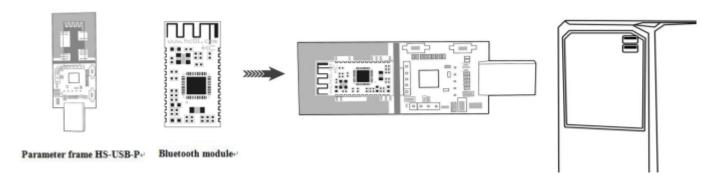
Put the HC-42 Bluetooth module into the HC-USB-P parameter frame, as shown in the figure. The module can be tested by plugging directly into the USB interface of the PC.
